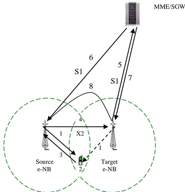
**Figure 1: Summary of the different steps of preparation, execution and completion HO process which performs by eNBs.**
