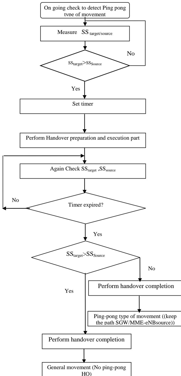
Figure 2 shows the ping-pong detection algorithm that presented in our work to reduce the number of ping-pong HOs in LTE networks
