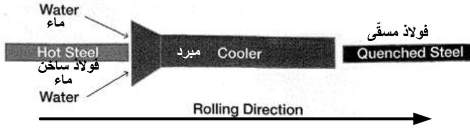
Representation of a functioning QTB cooler
