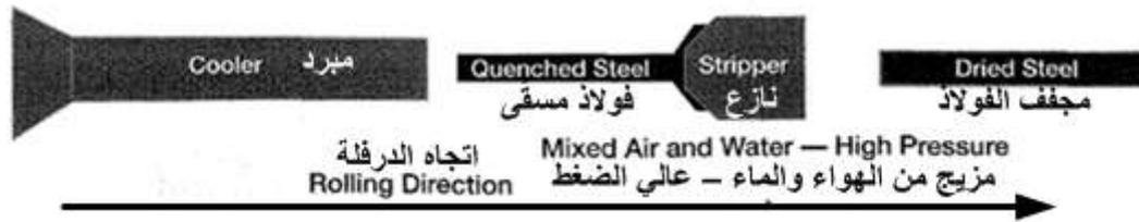
Representation of a functioning QT B stripper
