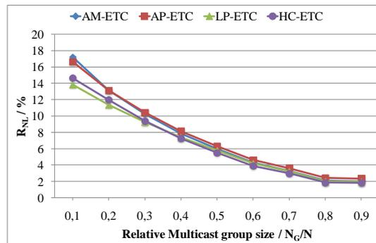
Fig. 8. Network load ratio of network B using estimated tree cost function.
