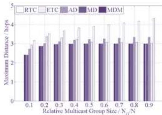
**Fig. 5. Comparison of the RP-selection methods for network A in terms of maximum distance.**
