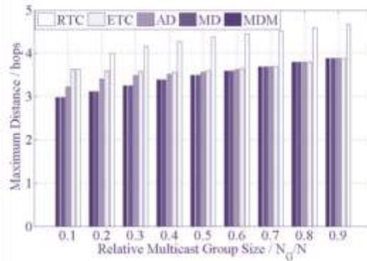
**Fig. 6. Comparison of the RP-selection methods for network A in terms of maximum distance.**
