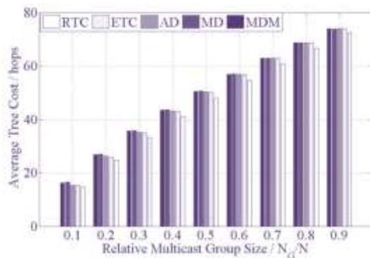
**Fig. 4. Comparison of the RP-selection methods for network B in terms of average tree cost.**
