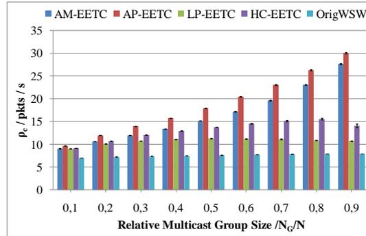
Fig. 13. Control load of network A using enhanced estimated tree cost function.
