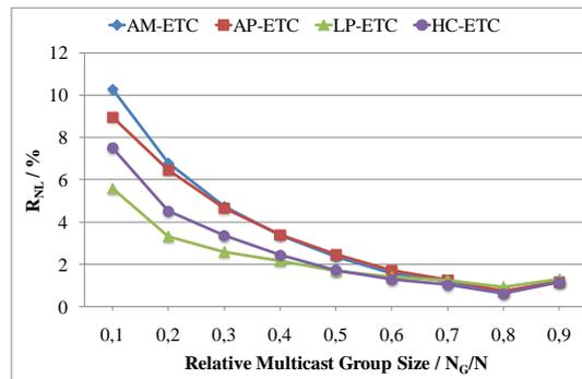
Fig. 7. Network load ratio of network A using estimated tree cost function.
