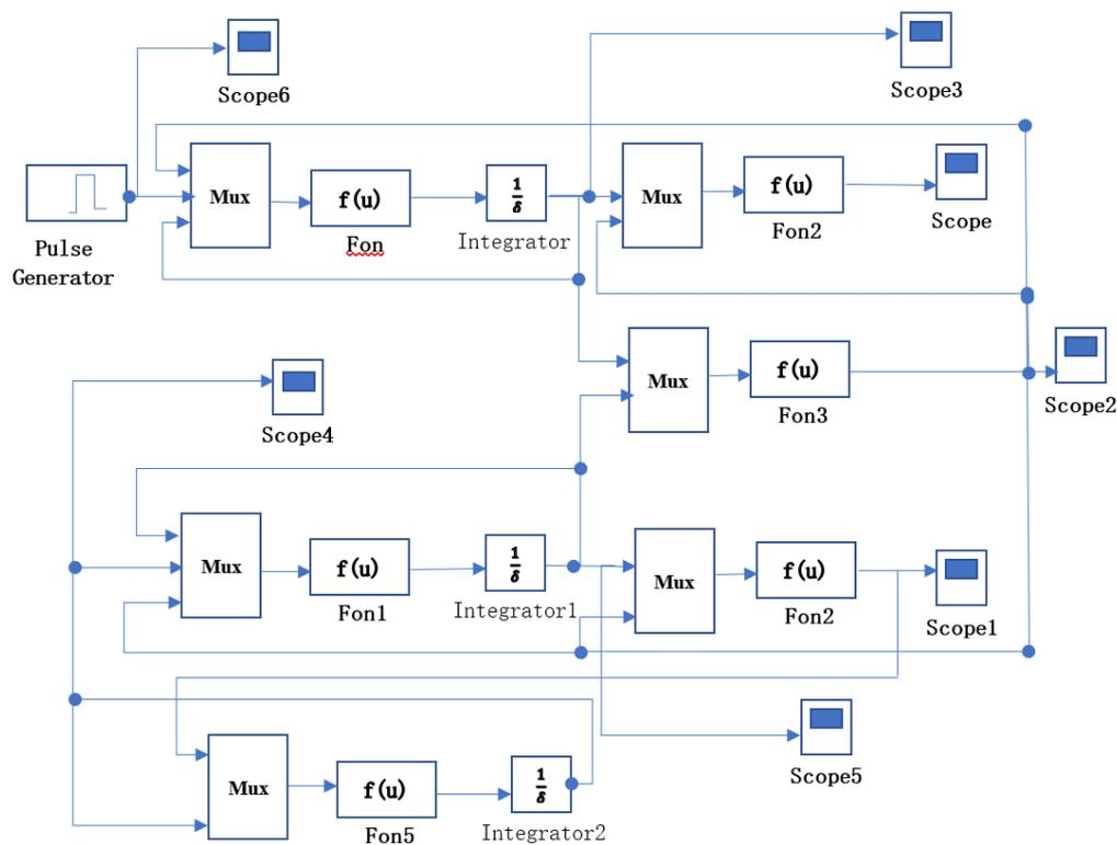
Fig. 4. MATLAB SIMULINK Simulation of pulse transformer based on flux linkage as state variable
