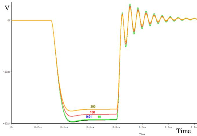
**Fig.10. effect of  $R_s$  on voltage drop of pulse Transformer response ( $R_s$ : 0.01, 10, 100, 200  $\Omega$ )**
