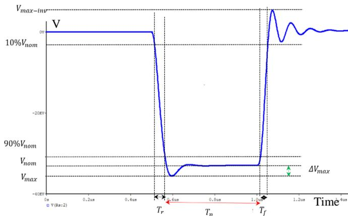
Fig.3. High-Voltage Pulse shape
