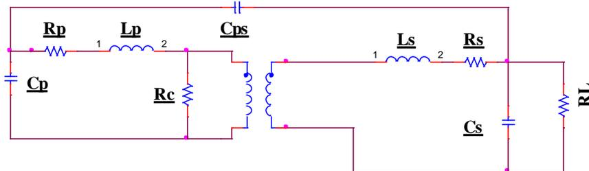
Fig.2. Basic scheme of IEEE equivalent circuit for Pulse Transformer.
