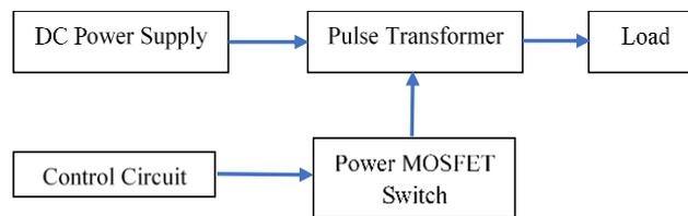
Fig.1. Block diagram of pulse modulators
