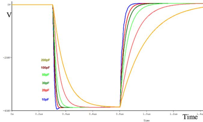
**Fig.14. effect of  $C_{ps}$  on rise and fall time of pulse Transformer response ( $C_{ps}$ : 10, 20, 30, 50, 100, 200 pF)**
