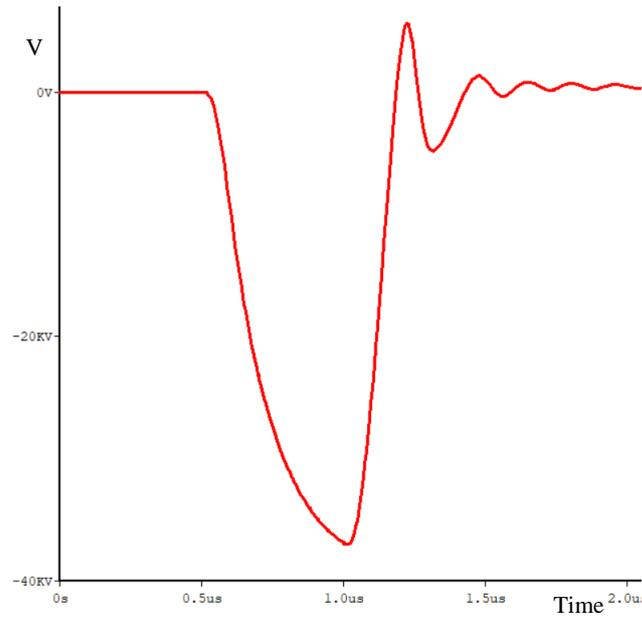
Fig.8. Waveform of  $V_s$  (periods of pulse transformer: 0.001,  $C = 2nF$  others parameters according to Table 1)
