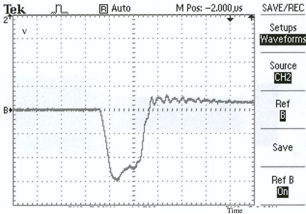
Fig. 19. Measured output high voltage applied to load which is unwanted
