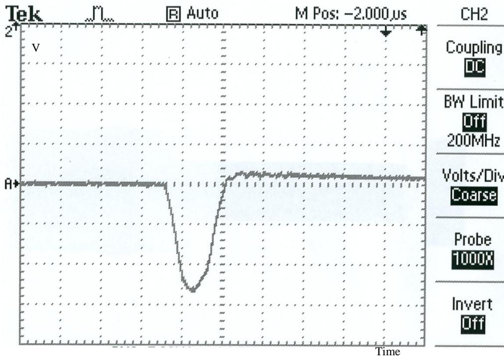
Fig. 20. Measured output high voltage 40 KV, with pulse width 500ns.
