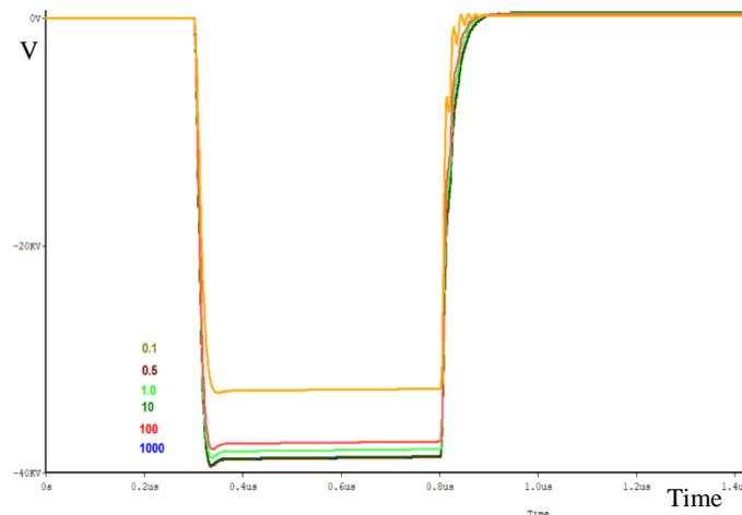
**Fig.11. effect of  $R_c$  on voltage drop of pulse Transformer response ( $R_c$ : 1000, 100, 10, 1, 0.5, 0.1  $\Omega$ )**
