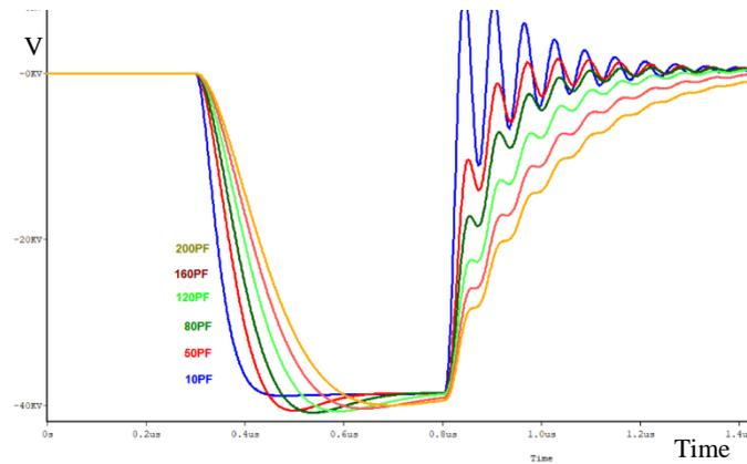
**Fig.13. effect of  $C_s$  on rise and fall time of pulse Transformer response ( $C_s$ : 10, 50, 80, 120, 160, 200 pF)**
