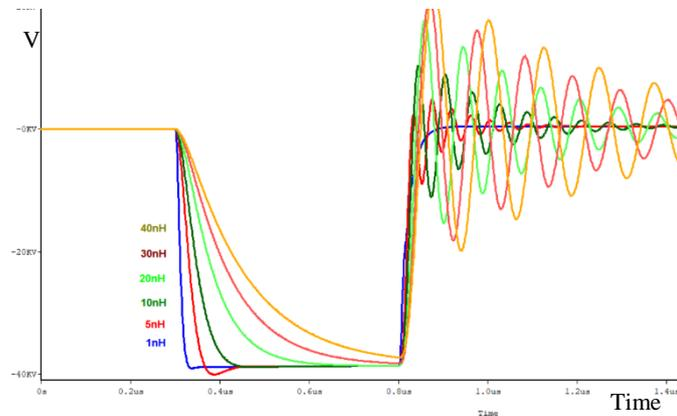
**Fig.15. effect of  $L_p$  on overshoot and back swing of pulse Transformer response ( $L_p$ : 1, 5, 10, 20, 30, 40 nH)**
