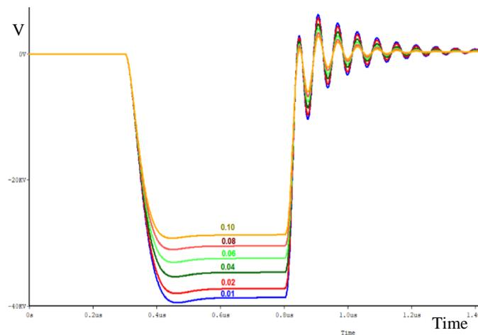
Fig.9. effect of  $R_p$  on voltage drop of pulse Transformer response ( $R_p$ : 0.01, 0.02, 0.04, 0.08, 0.1  $\Omega$ )
