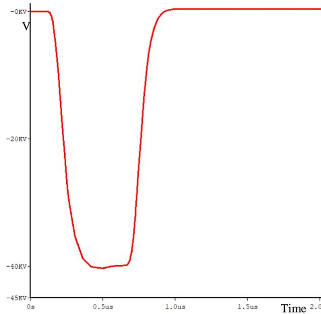
Fig. 5. Waveform of  $V_s$  (periods of pulse transformer: 0.001s)
