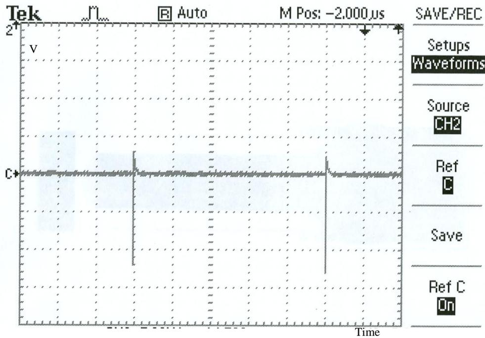
Fig. 18. Measured repetition of output high voltage applied to load (2KHz)
