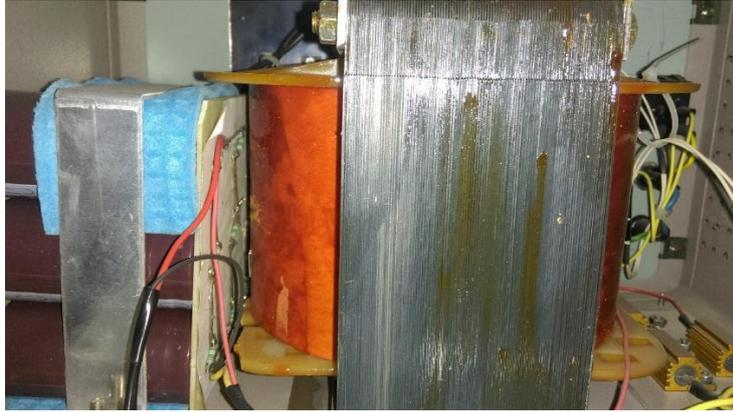
Fig. 17. Transformer double ferrite U93 core, 1 :10.
