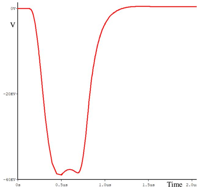
Fig.7. Waveform of  $V_s$  (periods of pulse transformer: 0.0002,  $x_{lp}=x_{ls}=1.24\Omega$  others parameters according to Table 1)
