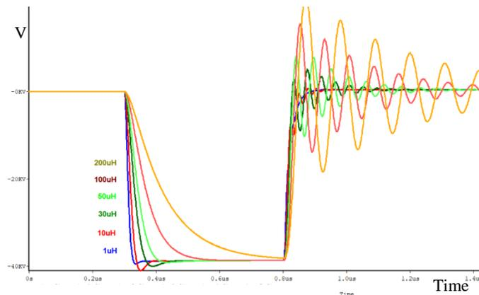
**Fig.16. effect of  $L_s$  on overshoot and back swing of pulse Transformer response ( $L_s$ : 1, 10, 30, 50, 100, 200  $\mu$ H)**
