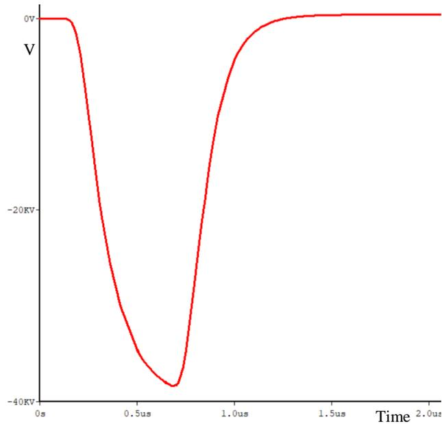
Fig. 6. Waveform of  $V_s$  (periods of pulse transformer: 0.0001s)
