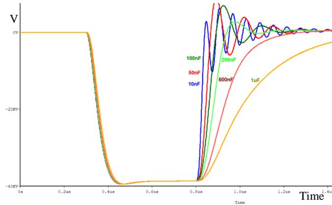
**Fig.12. effect of  $C_p$  on rise and fall time of pulse Transformer response ( $C_p$ : 10, 50, 100, 200, 500, 1000 nF)**
