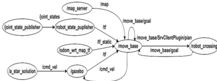
Figure (2): The data flow of the active nodes connection for the proposed A*
