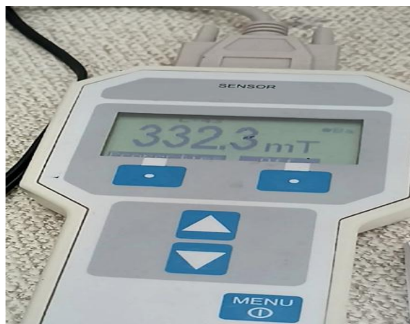
Figure 2. Measuring the magnetic field strength of a magnetization device.
