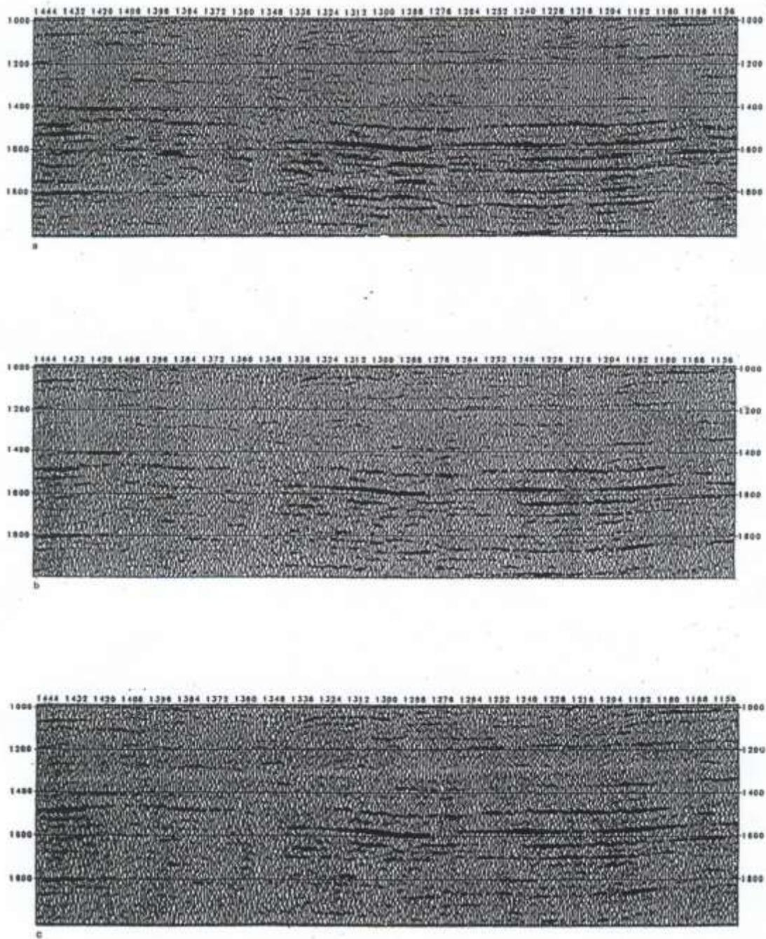
**FIG. 12.** Part of seismic section CH-81-36, CMPs 1151-1449. (a) Before deconvolution, multiples energy is strongly visible, especially around and below 1800msec time line. (b) After deconvolution with 32 ms gap length and 300 ms operator length applied. (c) After 600 ms operator length is applied. Multiples are suppressed and primary reflections have become more prominent.
