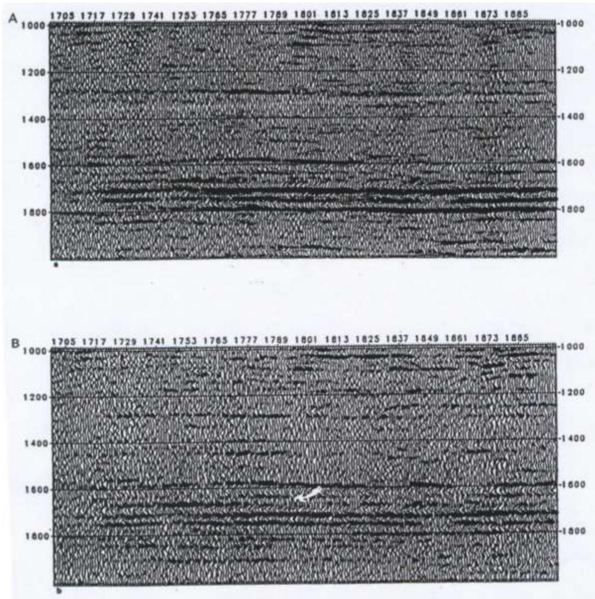
FIG. 5. Design gate of duration 1000 ms (1000-2000). Seismic section CH-81-37, CMPs 1700-1900. (a) Before. (b) After post-stack deconvolution of 32 ms gap length and 600 ms operator length applied.
