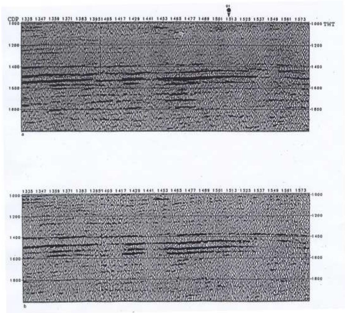
FIG. 11. Part of seismic section CH-81-37, CMPs 1330-1580. (a) Before deconvolution. (b) After post-stack deconvolution was applied with same parameters (and similar effect) as Fig. 10.
