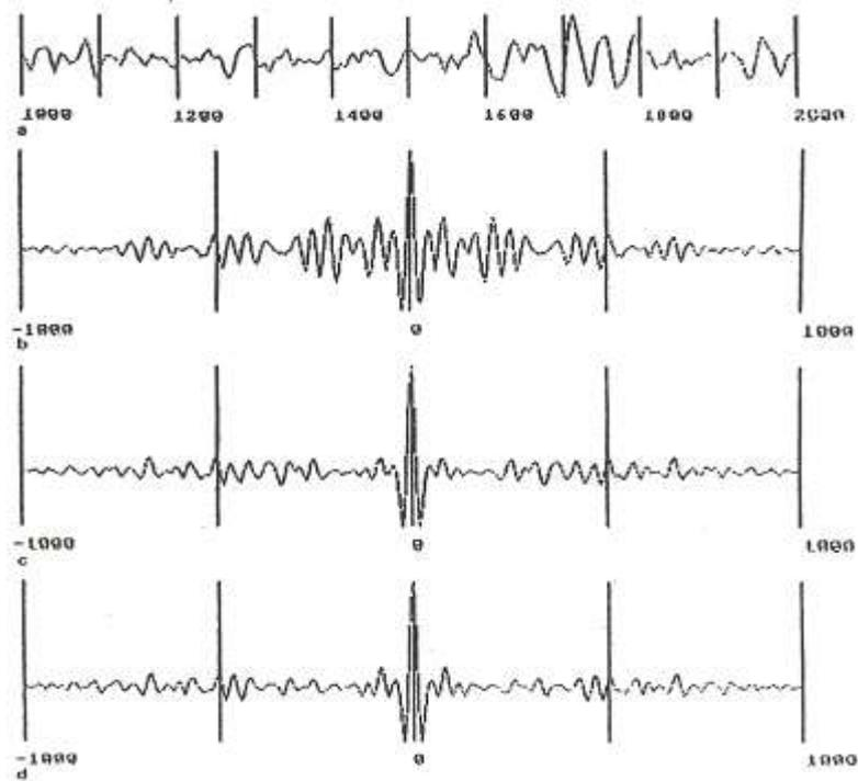
FIG. 2. Autocorrelation functions generated from a seismic section CH-81-37, CMPs 1790-1810, design gate 1000-2000. (a) (a) Input data trace window. (b) Function of input traces before deconvolution. (c) After deconvolution of 32 ms gap length and 300 ms operator length applied. (d) After 600 ms operator length applied. Refer to FIG. 8 for deconvolution effect in multiples attenuation.
