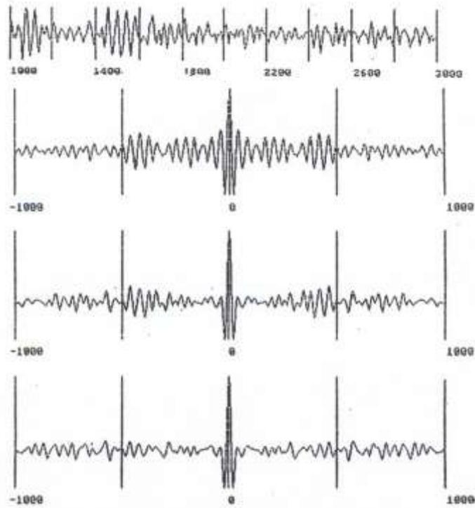
**FIG. 7.** Autocorrelation functions generated from seismic section CH-81-37, CMPs 2220-2240, and time interval 1000-3000 ms. Similar effect is shown regarding multiple attenuation to those used for deconvolution parameters computation in other parts of the sections.
