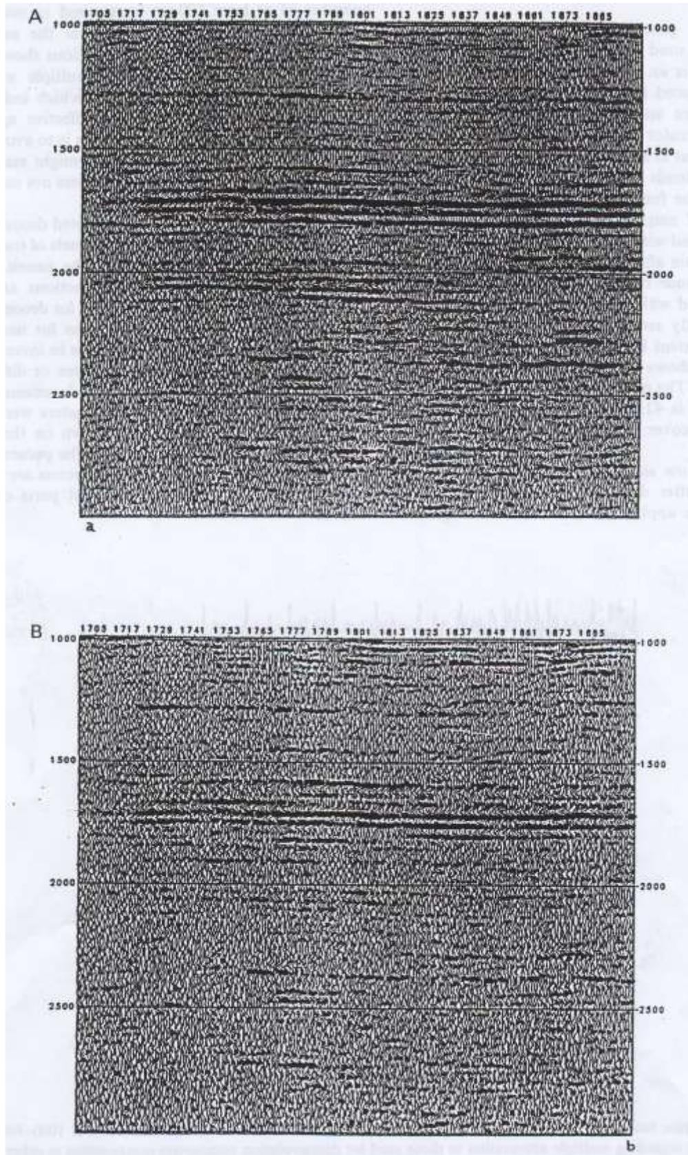
FIG. 6. Design gate of duration 2000 ms (1000-3000). Seismic section CH-81-37, CMPs 1700-1900. (a) Before. (b) After post-stack deconvolution of 32 ms gap length and 600 ms operator length applied.
