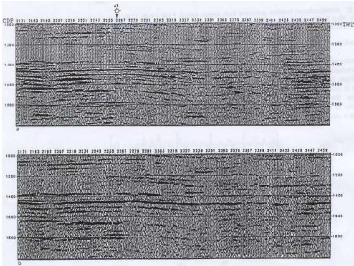
**FIG. 10. Part of seismic section CH-81-37, CMPs 2166-2466. (a) before post-stack deconvolution reflections are buried in multiple energy. (b) After post-stack deconvolution with 32 ms gap length and 600 ms operator length is applied. Significant amount of multiples related noise is removed and prominent reflections are more easily distinguished.**
