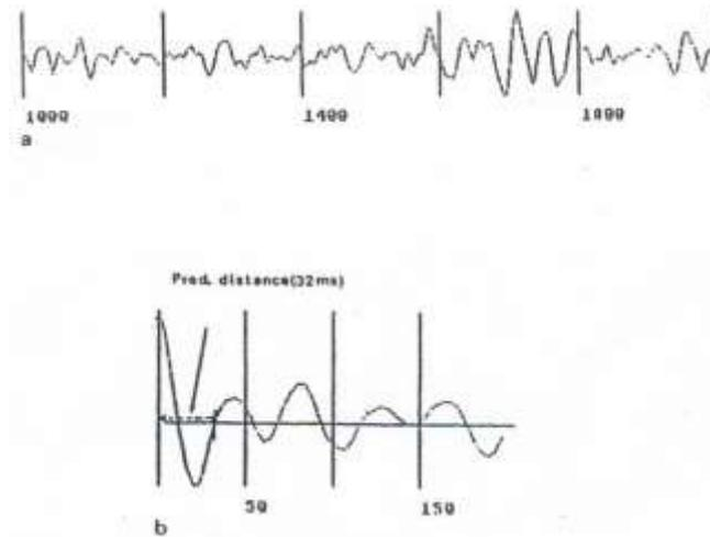
**FIG. 9. (a) Input trace from seismic section CH-81-37, and design window 1000-2000 ms. (b) Enlarged segment of the autocorrelation of the input trace showing the computation of prediction distance by applying the second zero crossing technique. Refer to Fig. 2b for multiple time duration.**
