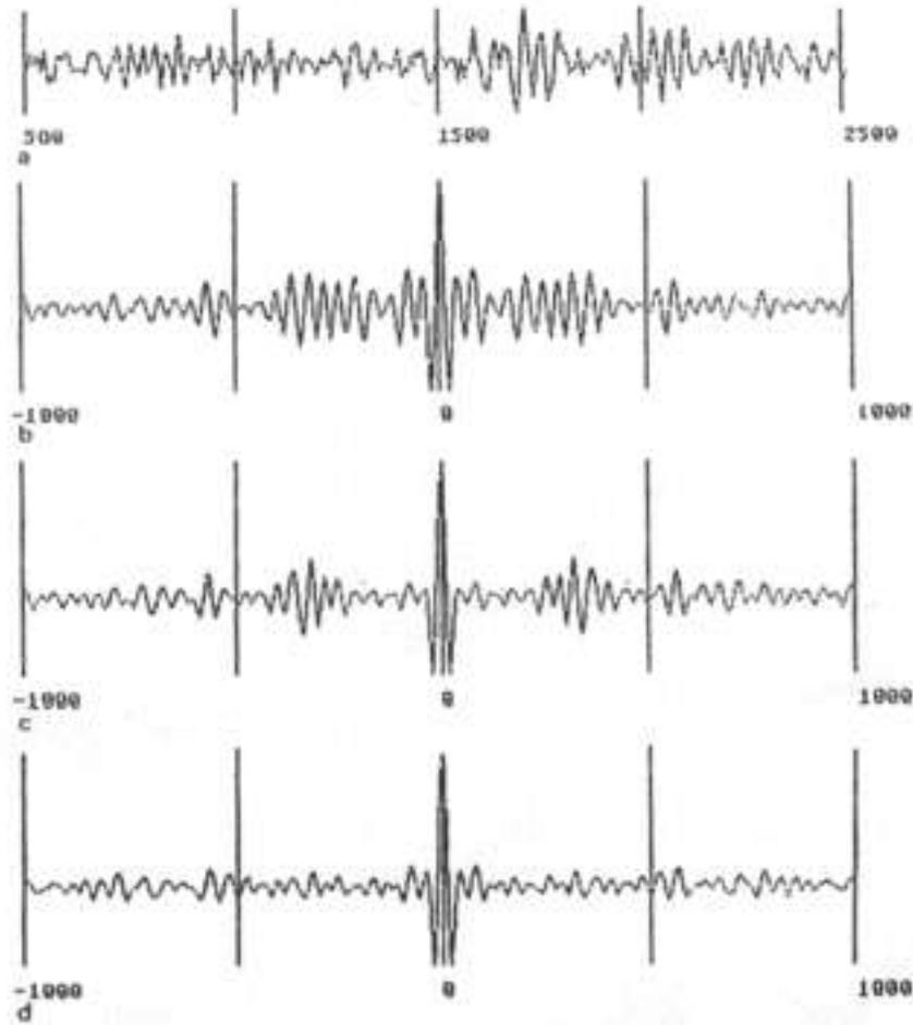
**FIG. 1. Autocorrelation functions generated from a seismic section CH-81-37, CMPs 1790-1810, design gate 500-2500. (a) Input data trace window from stack. (b) Function of input traces before deconvolution. (c) After deconvolution of 32 ms gap length and 300 ms operator length applied. (d) After 600 ms operator length applied. Refer to FIG. 7 for deconvolution effect in multiples attenuation.**
